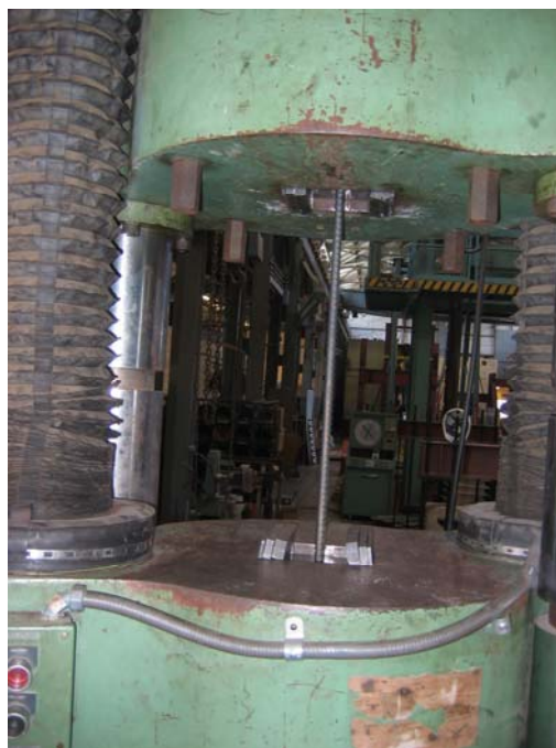
Figure 3.8: Tensile test of reinforcing steel
